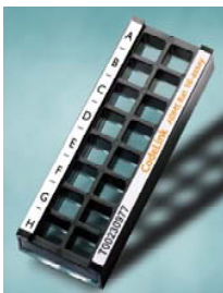
Fig 1. CodeLink multiassay bioarray chamber allows for processing of up to 16 arrays and samples in parallel on a single slide.
