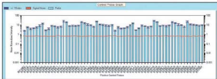
Figure A3.3. Typical sensitivity plot showing that normalized signal from each bacterial control probe is above noise for the set of control mRNAs spiked at an estimated mass ratio of 1:300,000. The noise level (the average mean background) for each probe is indicated by the red line.
